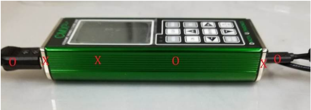
Photograph 6. ESD Test Points – Left of EUT
