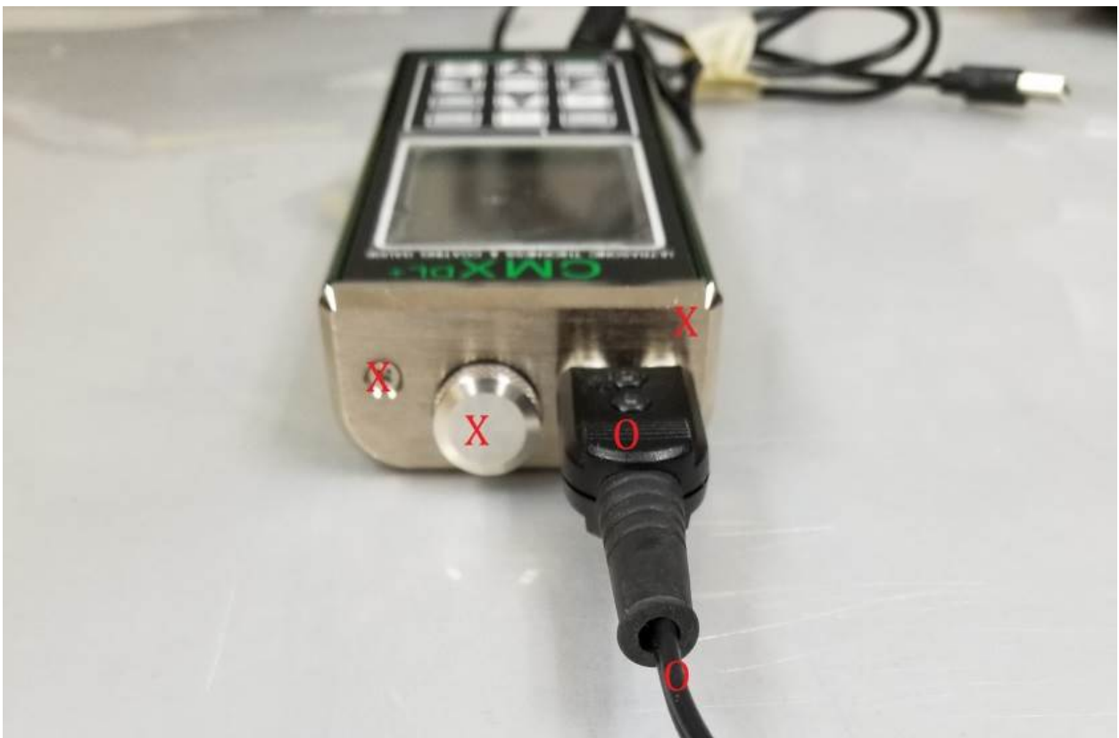
Photograph 7. ESD Test Points – Top of EUT
