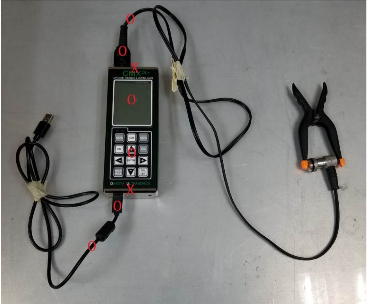
Photograph 3. ESD Test Points – Front of EUT
