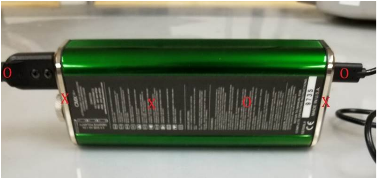
Photograph 4. ESD Test Points – Rear of EUT
