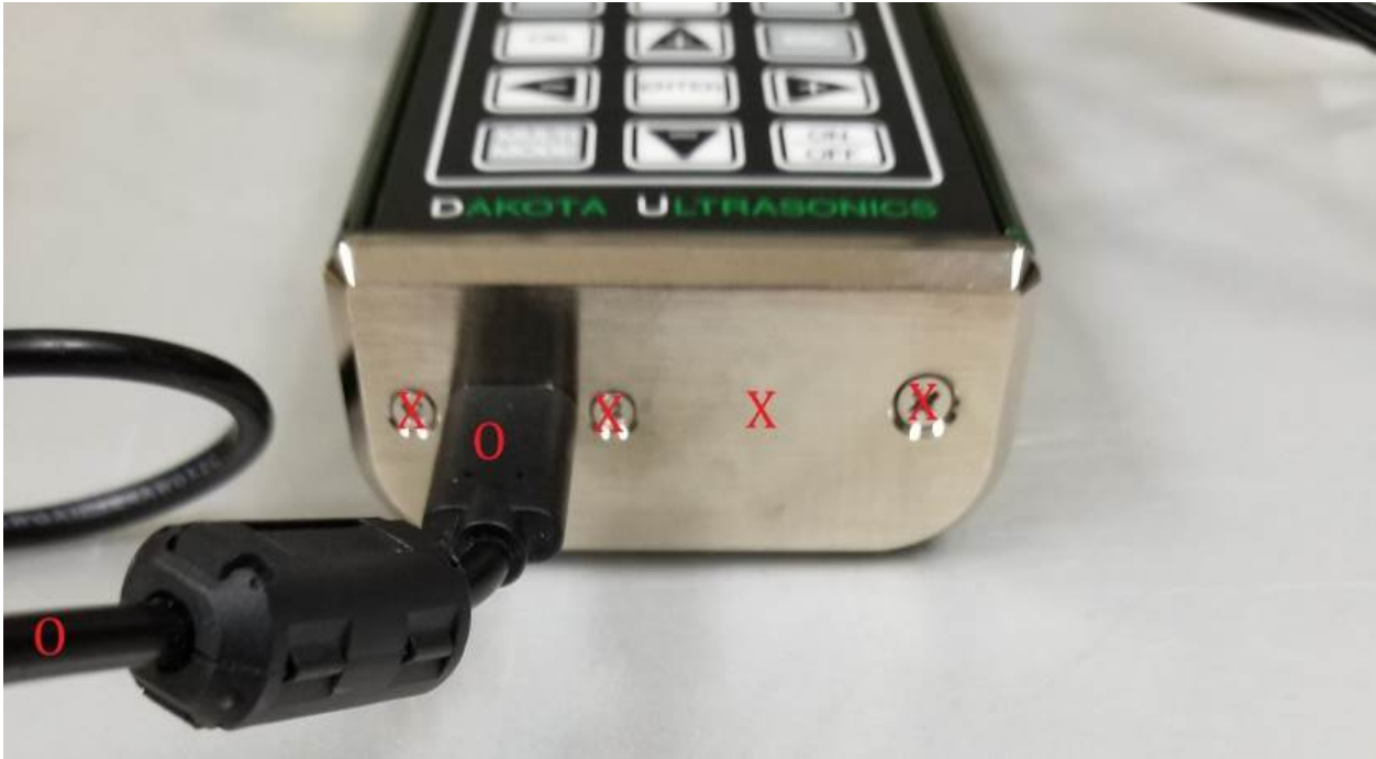
Photograph 8. ESD Test Points – Bottom of EUT
