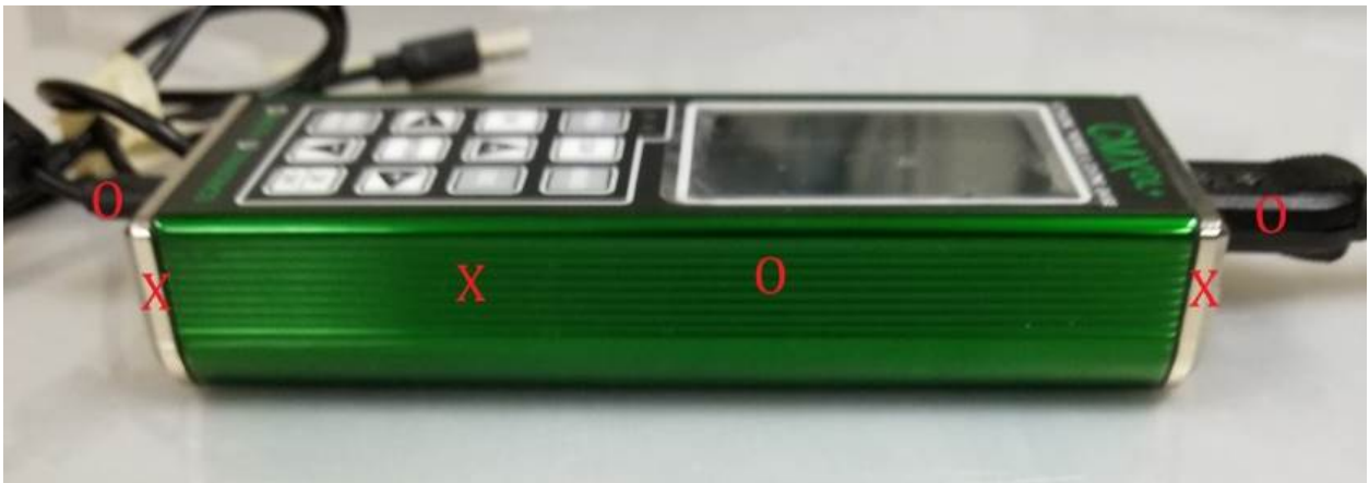
Photograph 5. ESD Test Points – Right of EUT
